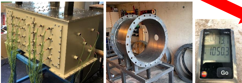
P-VHTTES-test module TESS 3B, ~100 kWh th , 1000 °C Commissioning in Q4/2022, enolcon laboratory
