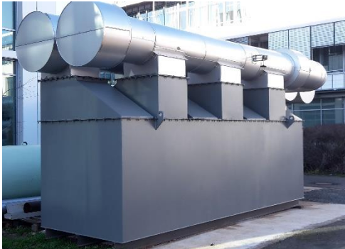
HTTES-test module TESS 3A, ~50 kWh th , 650 °C Commissioning in year 2020, enolcon laboratory and
