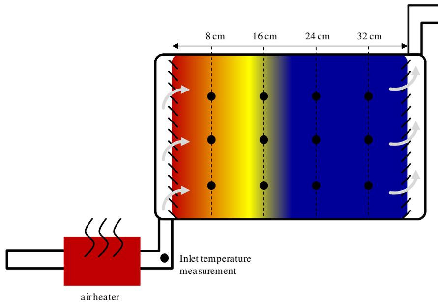
Fig. 5. Schematic layout of the test facility including the relevant measurement positions
