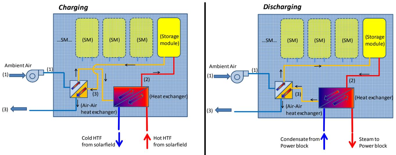
Fig. 1. Principal setup of the enolcon-HTTESS in charging (left) and discharging (right) mode
