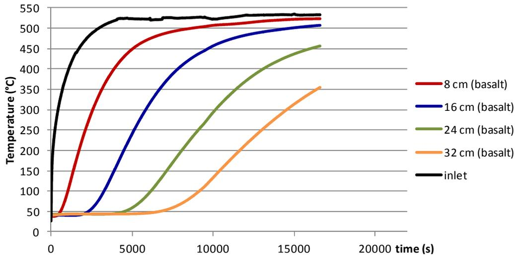
Fig. 8. Temperature behavior trough the packed-bed for 530 °C inlet temperature (*basalt gravel with 4 mm, air flow: 25 Nm<sup>3</sup>/h*)
