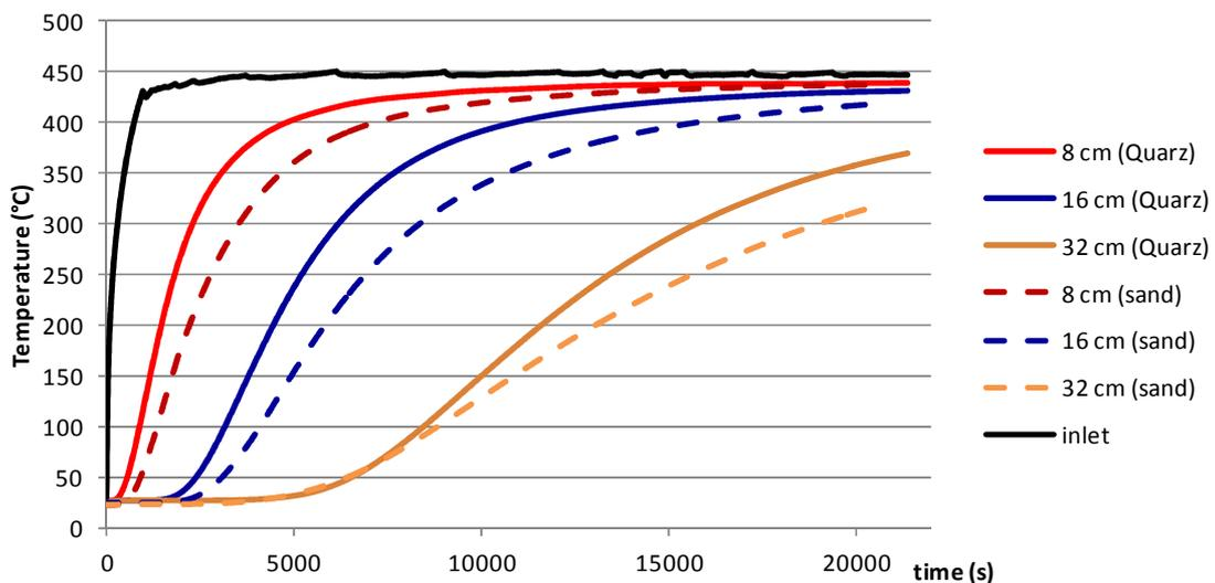
Fig. 7. Comparison of the temperature behavior through the packed-bed (quartz gravel with 2 mm, silica sand < 1 mm, air flow: 35 Nm<sup>3</sup>/h)
