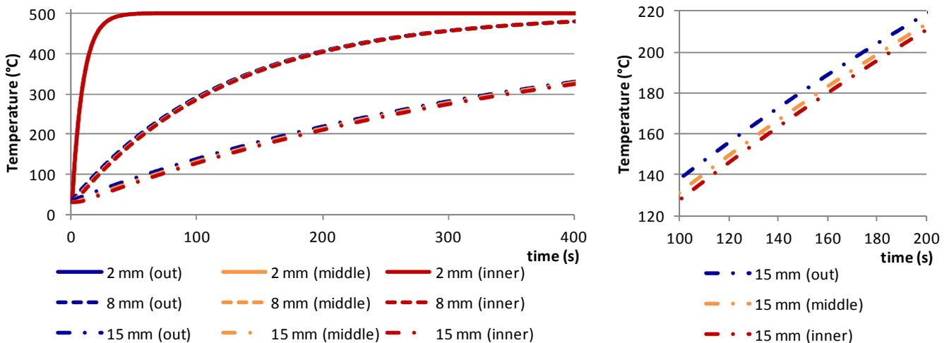
Fig.3. Modeled temperature behavior in different shells of a particular stone for three different radius (left), detailed view of the 15 mm radius (right)
