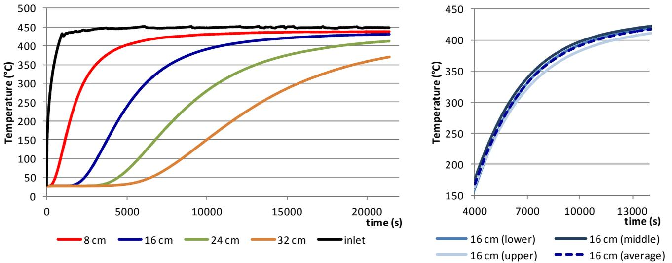
Fig. 6. Principal behavior of the temperature trough the packed-bed (quartz gravel with 2 mm, air flow: 35 Nm<sup>3</sup>/h)
