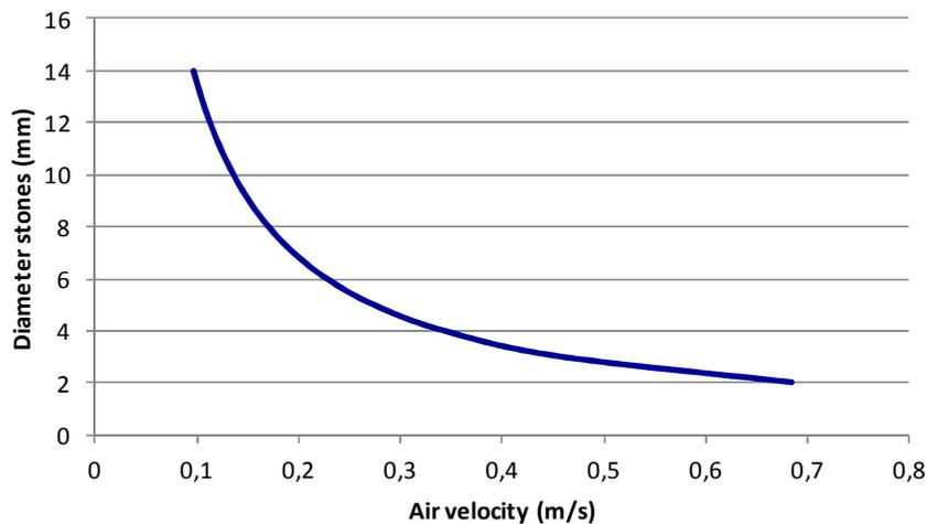
Fig. 4. Calculated Biot-Number of 0.1 based on the air velocity and the stone diameter, using (4)
