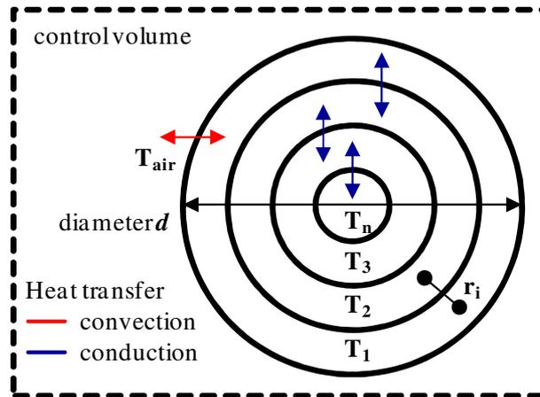
Fig.2. Used Shell-model for the simulation of the temperature behavior
