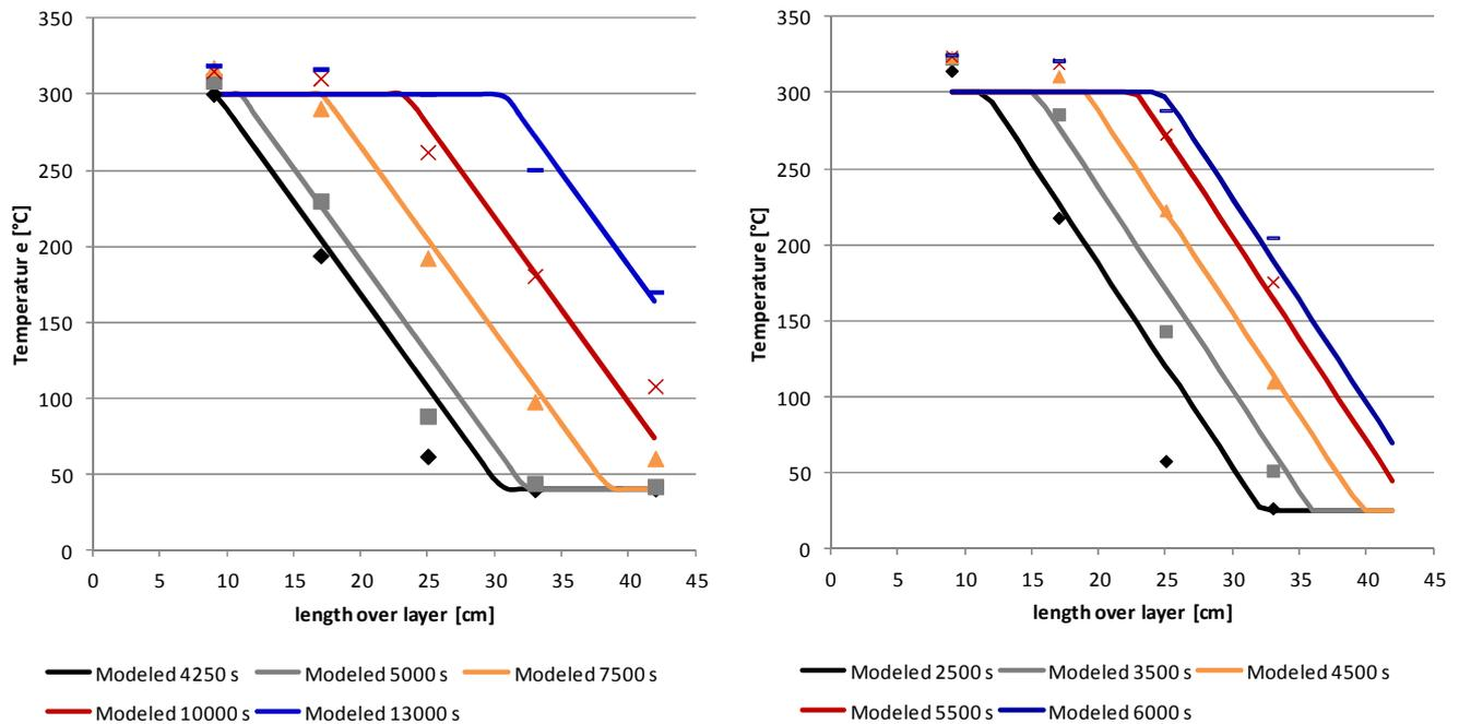
Fig. 9. Modeled thermocline through the packed bed (*quartz gravel, superficial velocity 0.12 m/s (left), 0.31 m/s (right)*)
