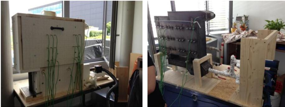
Figure 7: TESS002, left with isolation, right without isolation for first functional tests
